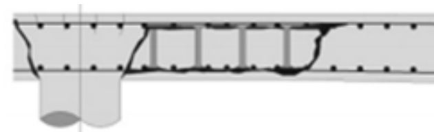
Delamination of concrete core
