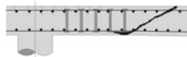
Failure outside shear- reinforced area
