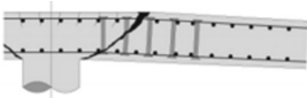
Failure within shear-reinforced area
